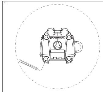
Check base is located away from objects that will obstruct the movement or removal of the ROKK Body and mark fixing positions.
