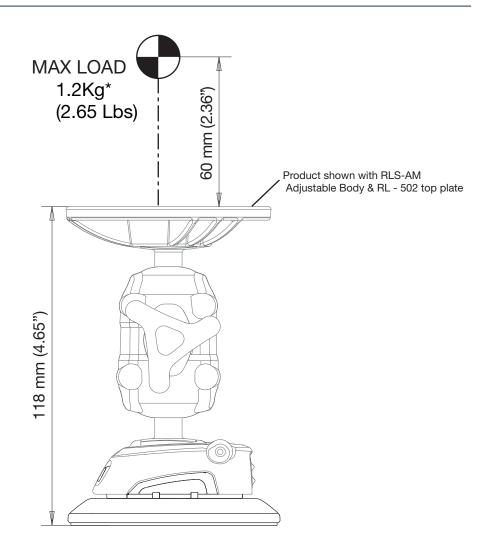
\*assuming product is installed in a dynamic environment where accelerations of up to 6g will be experienced
